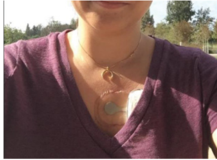
Fig. 1. Woman with heart condition wearing a chest-worn heart monitoring device. The device protrudes from the chest and is visible through most clothing.
