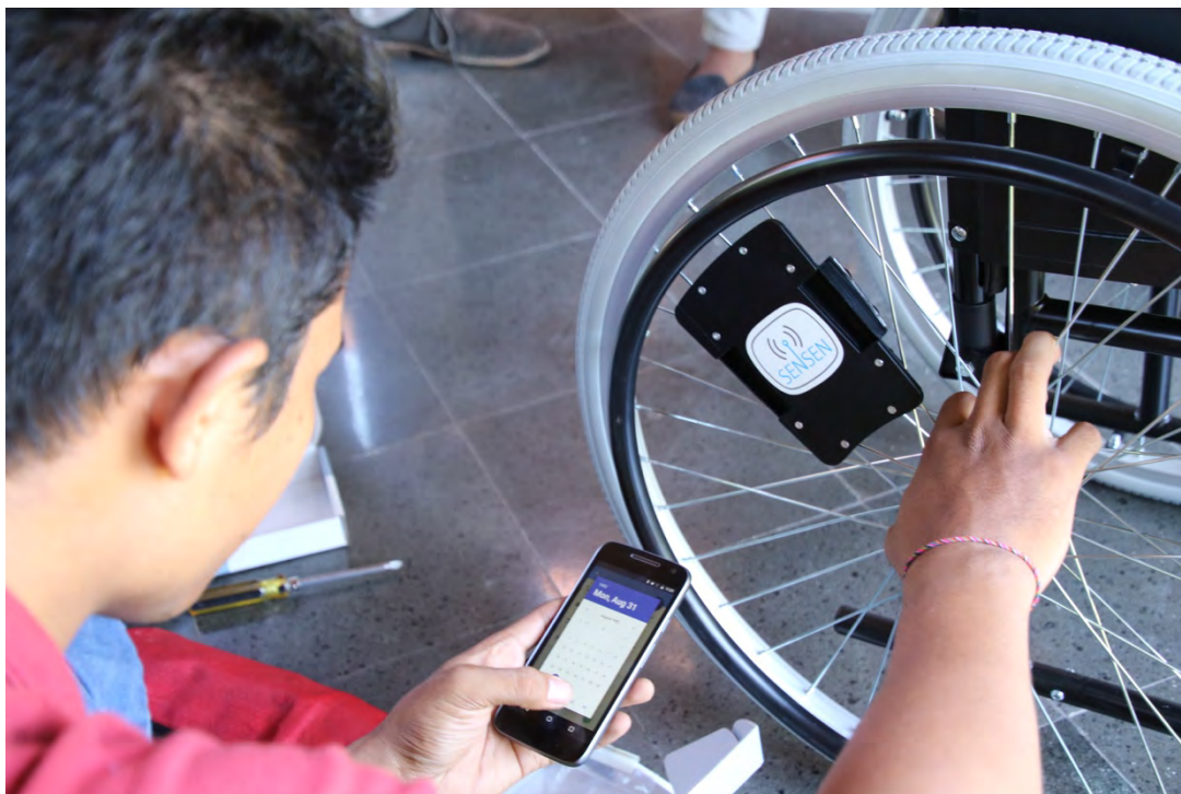
Figure 1. Numerator installing and configuring data-logger in participant's wheelchair.
