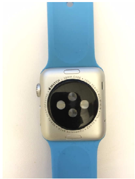
Figure 2: Sensors on Apple iWatch. The circles in the 3 and 9 o'clock positions are green and infrared LEDs. The ones in the 12 and 6 o'clock positions are photodiode sensors. (Image Credit: Shaun Kane)
